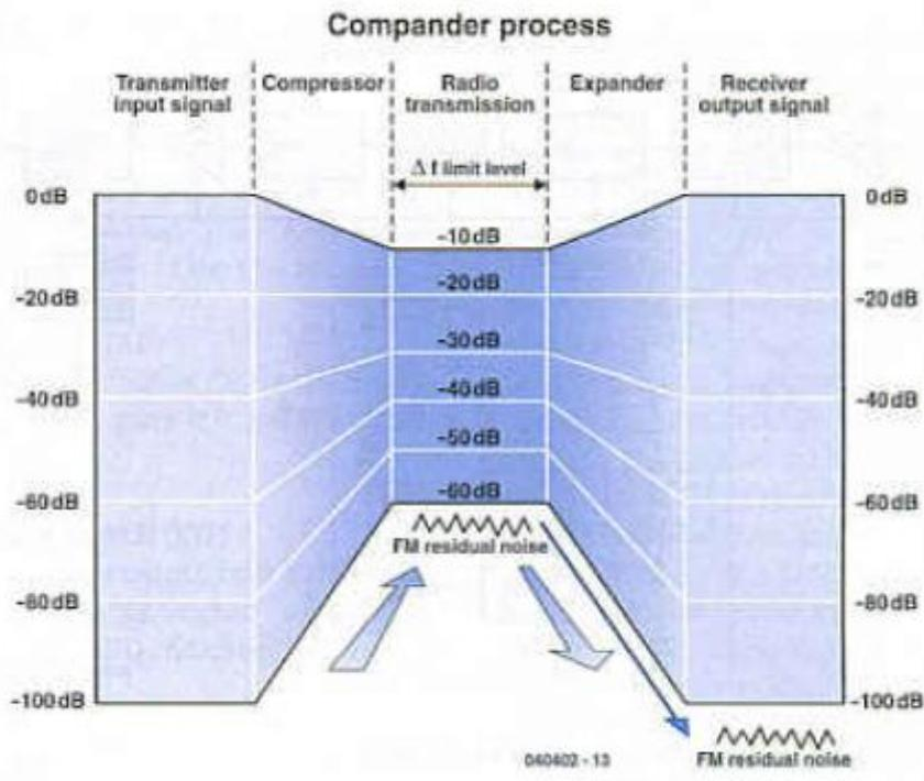
Figure 1. Use of a comander for noise reduction.
