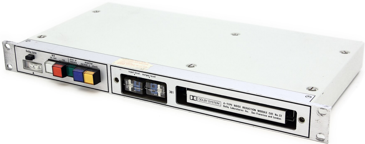
A Dolby 361 A-type noise reduction module(CAT. 22)
