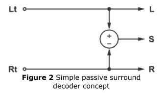
The simplest form of surround decoder subtracts the Rt signal from the Lt, as shown in Figure 2. If only an S signal is present at the encoder, the signals in Lt and Rt are identical but of opposite polarity. When these signals are subtracted in the passive decoder, they create the surround output signal as desired.
