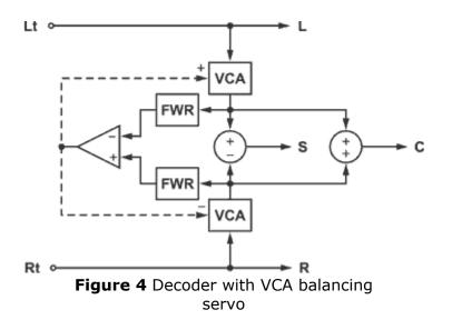
To automatically maintain the balance of the two signals feeding the subtraction stage under dynamically changing signal conditions, a feedback "servo" circuit
