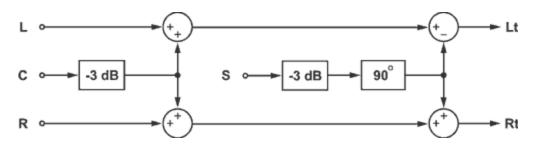
Figure 1 Simple four-input encoder concept
