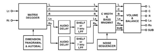
Figure 5 Basic decoder system block diagram
